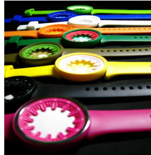
Photo 3: Cast parts from a silicone mold
