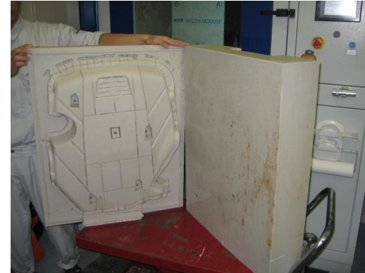
Photo 6: Silicone mold for nylon casting
