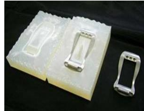
Photo 2: Silicone mold & prototype
